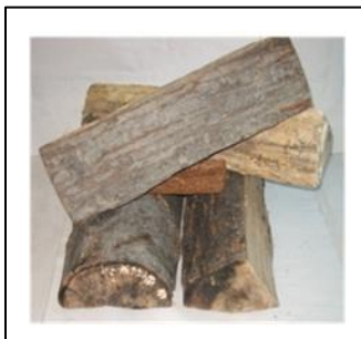
Figure 4-2: Recommended Wood Configuration
