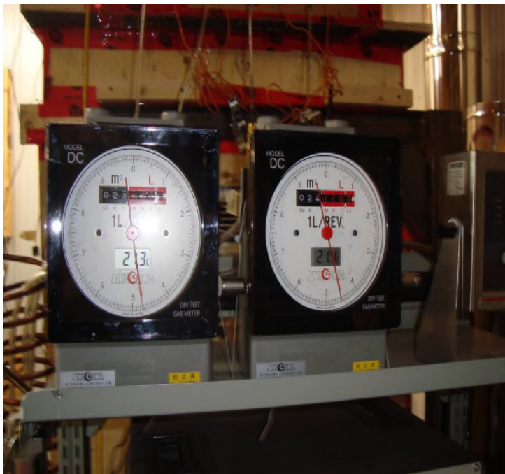
Picture 11: Dry gas meter
