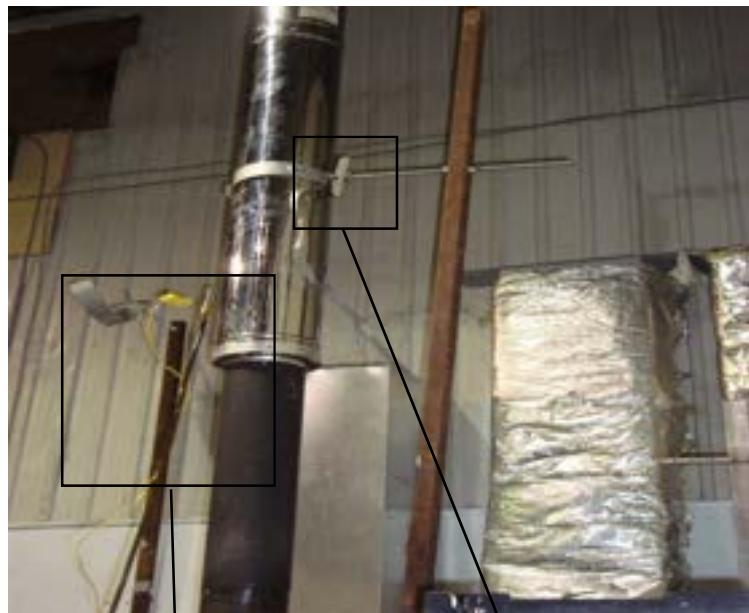
Picture 3.1: Gas analysis and temperature probe
