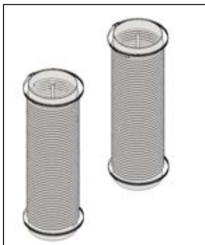
Figure 3-28: CAC8 Ducts with Worm Gear Clamps
