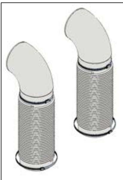
Figure 3-29: Installation of 90° Elbows on CAC8 Ducts
